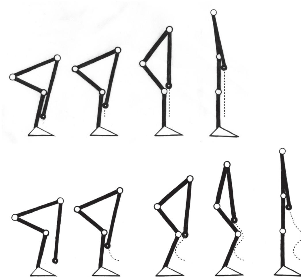
**Figure 4-19.** The work done against gravity is purely vertical displacement because the force of gravity acts vertically. Any other movement of the bar is horizontal motion that does not represent work done against gravity and is therefore effort spent inefficiently.
